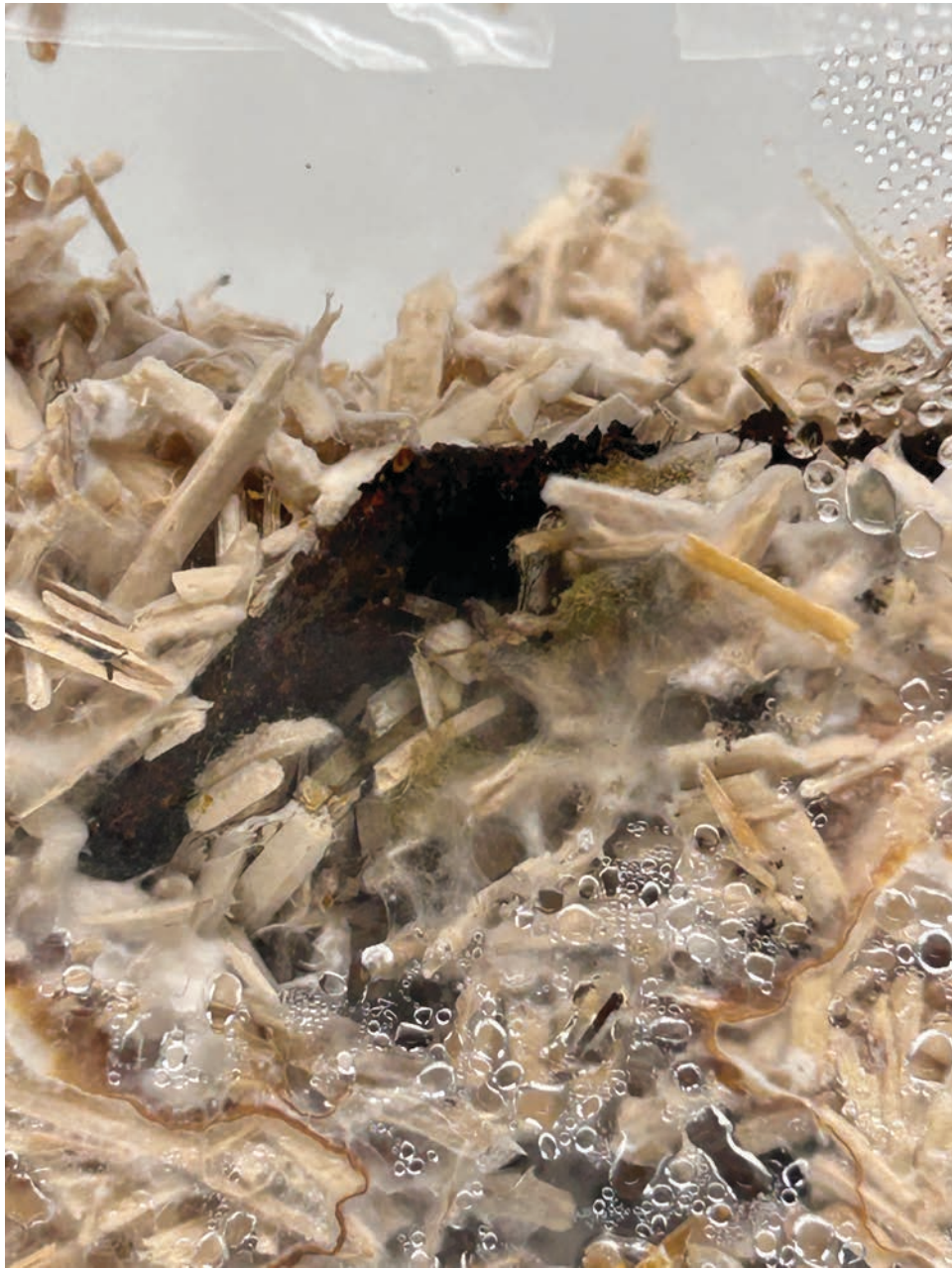
Detail from the mycelium box with corroded steel - the mycelium was growing around the metal piece.
